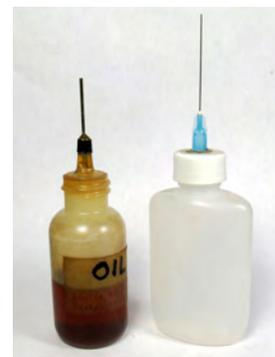
I use the small one on the left for oil when I'm sawing or drilling harder metals like steel. And I use the bottle on the right from a plastics store for the fast drying glues used to join pieces of acrylic.
