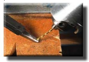
I solved the problem by forming a groove at the end of the jaw that would grasp the ring gently without scratching it. Use a triangular file or cutoff disk to cut the grooves about 1.5 mm back from the tip. Then to make the grooves round so they grasp the wire without distorting it, close the jaws and run a drill through the opening formed by the two rough grooves. Start with a small drill and follow up with a drill just
