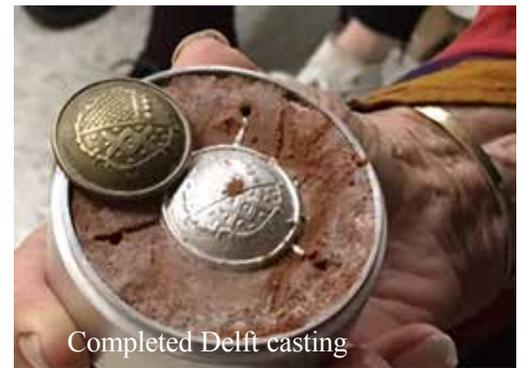
escape while metal was poured in. Finally, Brad put the two halves of the mold together and poured melted metal into the cavity through the funnel. Once the metal had solidified, he opened the mold and removed the piece.
