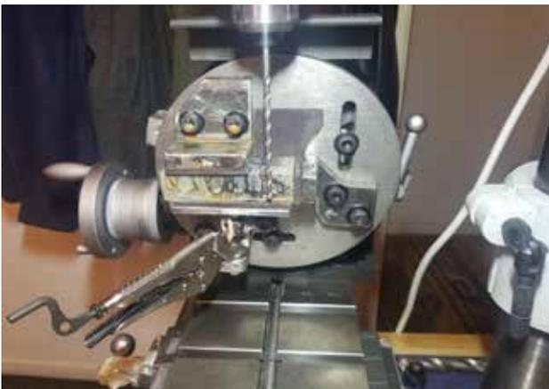
*A close up of the scratch built drilling clamp fixture, with the splash back removed to provide fuller view. Note that the stone block is uncovered on the top and left. The fixture, allowing holes to be drilled in two directions, that will intersect at a desired point within the stone.*
