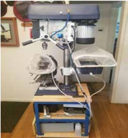
*An overview of Cokin's "3 square foot workshop." The grinding station is stored out of the way on the right, and may be swung around in front of the drilling station on the left, to be coupled with the drill motor.*
