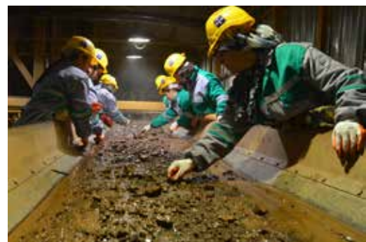
In Turkey, workers along a conveyor belt picked rough gems out of bauxite production. Image by Milenyum Metal Madencilik AS
